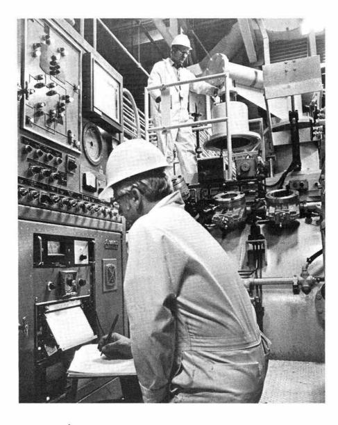
INSIDE THE MELT LAB, Joe Dal Perto (5833), foreground, checks the immersion thermocouple readout to determine temperature inside the melt crucible. Bob Fisher (5833) operates vacuum charging crane.
